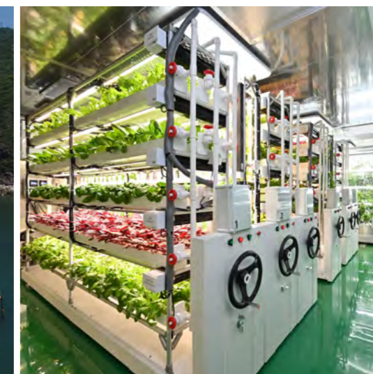
Mobile Hydroponic Cultivation System
